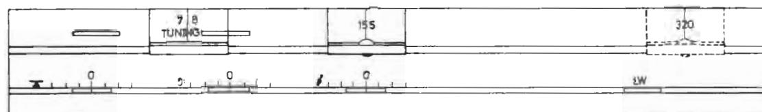
Alignment of LW signal-frequency circuits. 230 kHz: 15  $\mu$ V/ 10 dB s/n.
