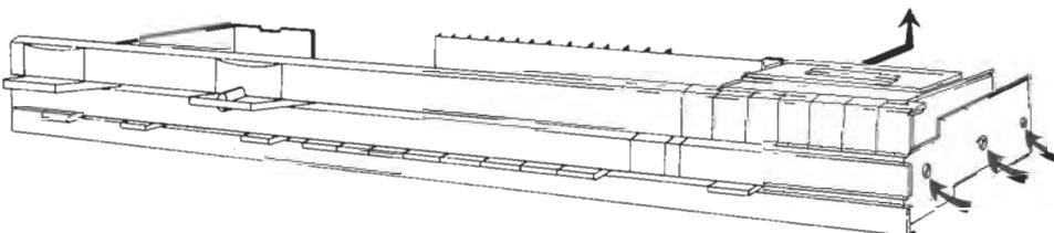
**Dismounting of Front Profiles / Demontierung der Frontprofile**
