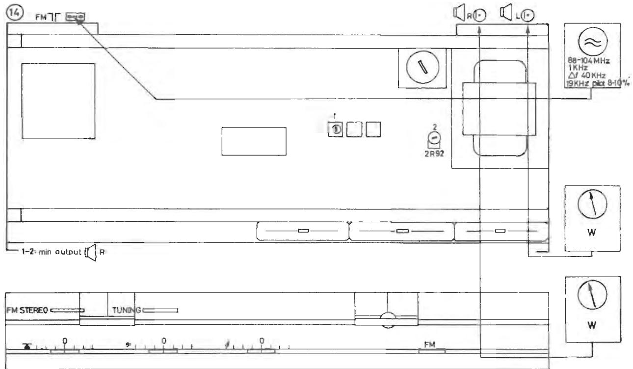
Adjustment of channel separation. Left channel modulated.
