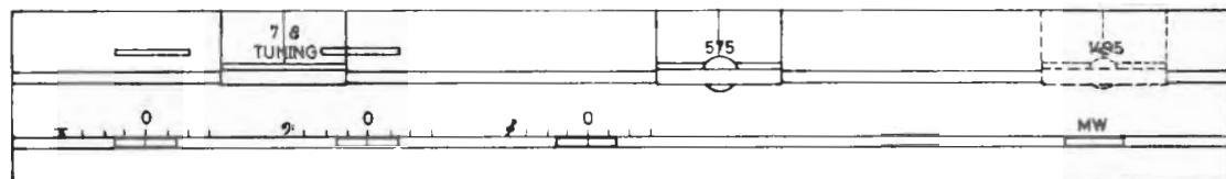
Alignment of MW signal-frequency circuits. 1007 kHz: 20  $\mu$ V/ 10 dB s/n.
