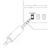
Headphone Socket. This socket is located on the front panel of the BEOCENTER 3500. It is intended for headphones equipped with a jack plug (impedance between 500 and 10.000 ohms). A suitable B&O jack plug carries the type no. 7222022.
