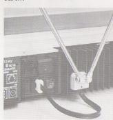
purchase a Bang & Olufsen type 8902010 FM aerial. It goes into a holder on the back of the set, and the cable plugs into the 240-300-ohm socket.
