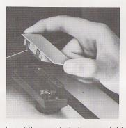
Insert the counterbalance weight in the rear section of the pickup arm.
