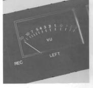
so that VU 0 dB corresponds to the standardized Dolby level (200 pWb). Without Dolby, recording can take place until 2 dB at the VU-meters (250 pWb at 3% distortion).
