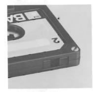
On an unrecorded tape cassette, these apertures are closed by a tongue which allows operation of the RECORD button.
