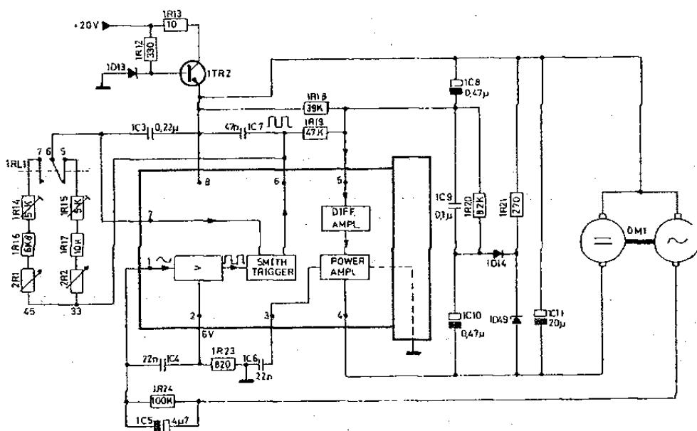
The turntable is driven by a tacho-controlled DC motor. A generator in the motor furnishes an AC voltage whose frequency is dependent on the motor speed.
