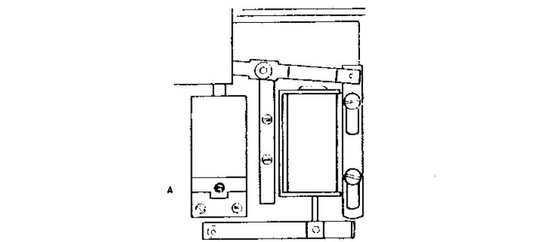
Adjust the valve A so that the pickup lowers at a uniform rate of speed.
