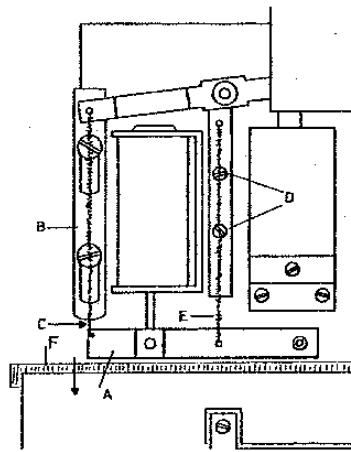
Loosen screws D. Pull arm A in the direction of the arrow until the separation between arm A and arm B at the point C is 1 mm. Move the magnet coil until the armature is the whole way down, and tighten screws D.
