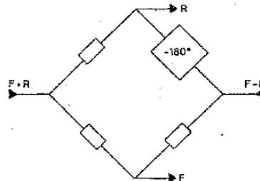
The principle of the matrix is, in one case, to add the two signals together to produce the front signal and, in the other, to subtract them so as to obtain the rear signal.
