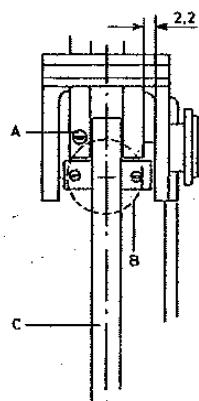
Place the pickup arm in the bearing bracket so that the middle line C of the pickup arm is located in the centre line of the shaft B with an accuracy of  $\pm 0.2$  mm. Adjustment is performed by loosening screw A and sliding the pickup arm to one side or the other and thereafter retightening the screws A. Use a gauge (e.g. a 2.2 mm drill) placed as shown in the sketch.
