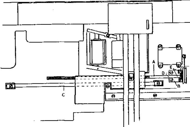
Adjust the spindle A so that it is parallel with the rod C both in the vertical and horizontal planes.
