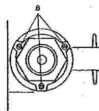
Turn the transit screws to lock the floating chassis.
