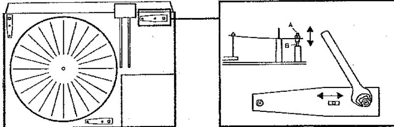
Loosen the transit screws so that the chassis floats.
