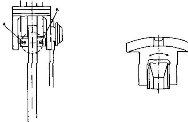
By loosening the screw A and tightening the screw B, or vice versa, adjust the turning of the pickup arm so that its top side is parallel with the rods. A check can be made by means of a spirit level with the Beogram placed on a horizontal support.
