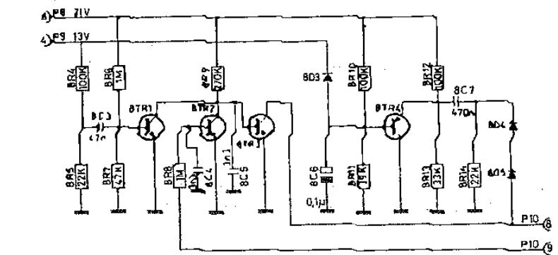
While a record is being played, 8TR2 is forward biased, the collector is low and 8TR3 reverse biased. Because of the voltage divider 8R4 · 8R5, 8C3 is charged to approx. 6 volts. When a change to another program is made on the remote control unit, the 13-volt potential at pin 4 of P9 disappears, 8C3 will discharge through 8R5 and 8R7, causing 8TR1 to be reverse biased.
