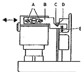
The pickup arm should be adjusted to be parallel with pins A in tool 3624009.
