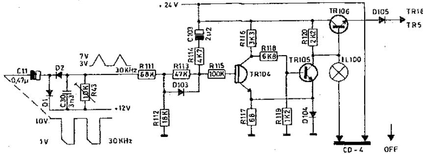
When a stereo record is played, 12V is present at the anode of D2. TR104 is forward biased, the collector goes low, and TR105 is reverse biased. The collector of TR105 goes high, and the CD-4 indicator IL100 is off. The high level at the collector of TR105 provides forward bias for TR106.
