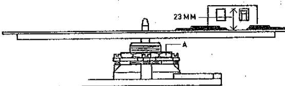
Loosen nut A at turntable bearing and adjust the height of the bearing so that the separation between turntable and detector arm is 23 mm.
