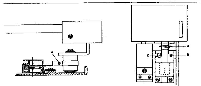
The diaphragm is adjusted by loosening the screw A and turning it on the pivot.
