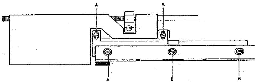
With screws A loosened, the position giver angle can be adjusted so that the position giver runs parallel with the photo resistor housing.
