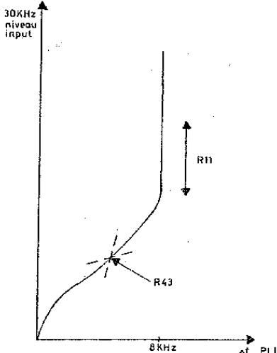
The carrier detector serves the purpose of limiting the lock-in range of the PLL if 30 kHz carrier drops out. Limiting follows the curve shown, the slope of the curve (level range) being adjusted with R43. R11 is used for selecting the 30 kHz level at which regulation starts.
