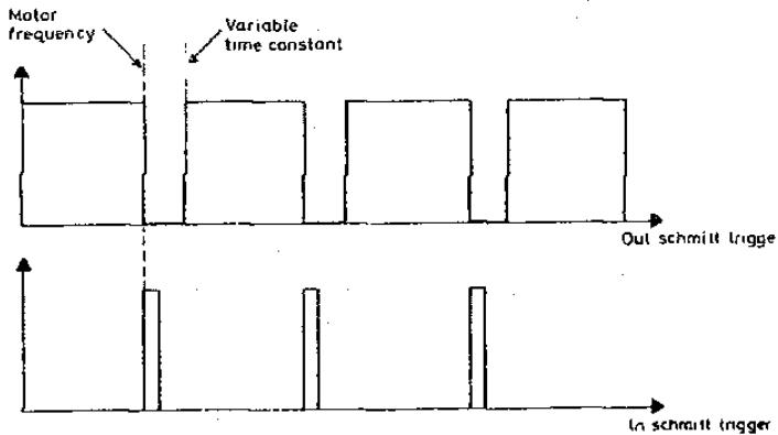
The output signal of the Schmitt trigger (pin 6) is integrated across 1R19 - 1C8 and fed to pin 5 which is a differential amplifier. The integrated signal at 5 will be a DC voltage which varies with the motor speed. This DC voltage is fed via the differential amplifier to a power amplifier. The power amplifier is connected as a variable resistor to chassis potential. 1C10 - 1C9 - 1R20 provides negative feedback for the power amplifier (see sketch), preventing "overregulation".
