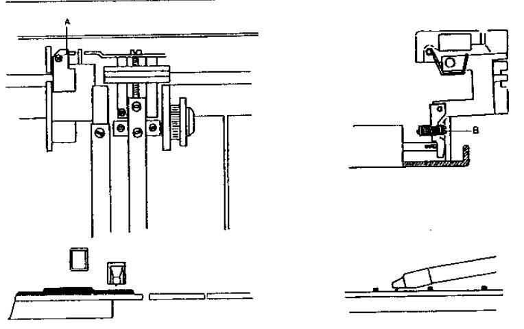
Loosen the screw A.
