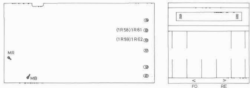
Connect vacuum-tube voltmeter at point MR. Depress FO button and adjust voltage at point MR to 5,5 V, using 1R61 (1R58).
