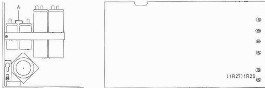
Connect LF vacuum-tube voltmeter and oscilloscope at point A so that measurements will be made with respect to chassis (zero) potential.
