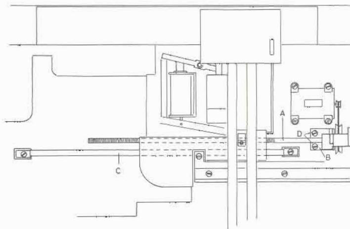
Adjust spindle A to be parallel with rod C.
