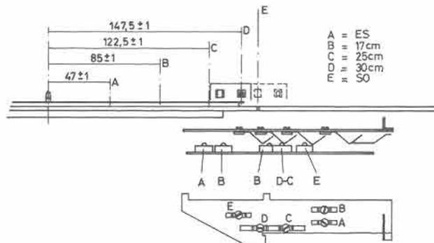
The horizontal placement of the springs should be made so that they will actuate their respective contacts during slide transport when the pickup is spaced from the middle of the centre pin by the amount stated on the sketch.
