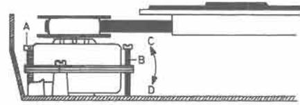
The drive motor should be adjusted so that the belt runs in the middle of the pulley and the belt face on the turntable.
