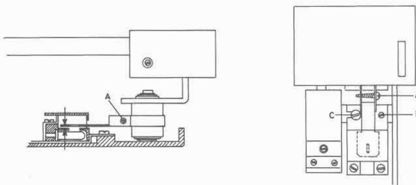
To adjust the shutter, loosen screw A and slide it on the arm pivot.
