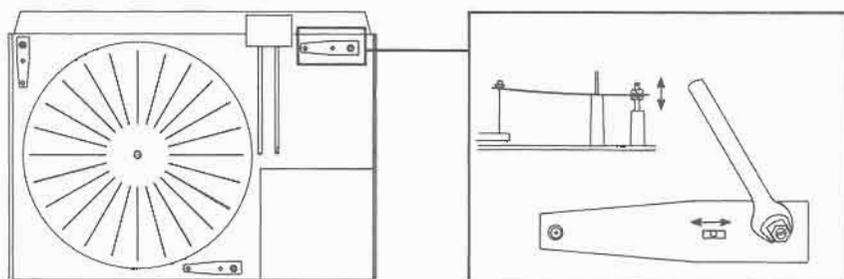
By means of the suspension springs adjust the chassis so that turntable is flush with the cover plate and so that the chassis is placed in middle of the transit screws.
