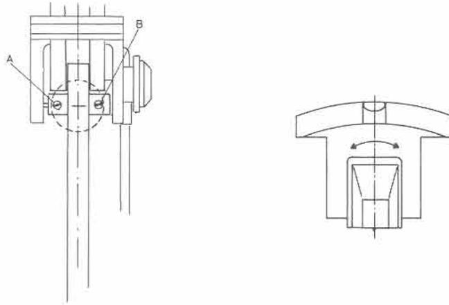
By loosening screw A and tightening screw B or vice versa adjust the rotation of the pickup arm so that its top side is parallel with the rods. Use a spirit level for checking this adjustment.
