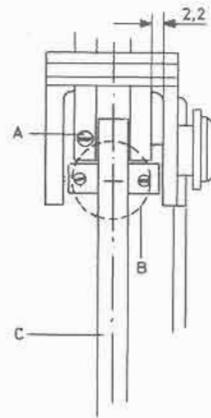
Place pickup arm in pivot bracket so pickup-arm centre line C is located in the centre line of the pin B with an accuracy to  $\pm 0,2$  mm. Adjustment is made by loosening screw A and sliding the pickup arm to one side or the other, thereafter retightening screw A.
