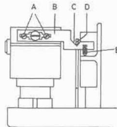
The pickup arm should be adjusted parallel with pins A in tool 3624009.
