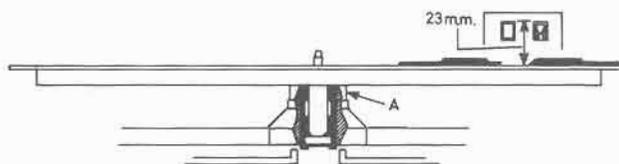
Loosen nut A at turntable bearing and adjust the height of the bearing so that the spacing between the turntable and detector arm is 23 mm.
