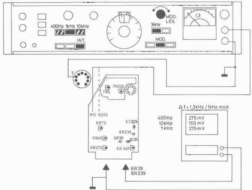
The dB values specified in the Adjustment Procedure refer to 0 dB = 1 V RMS.
