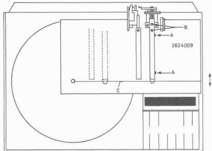
Adjust stylus force to 1 gr. Take off turntable. Run pickup arm in towards the centre.
