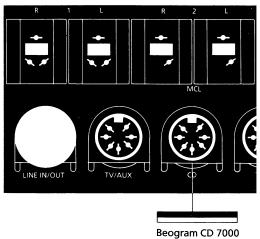
The digital output on the rear panel is intended for possible future digital equipment.
