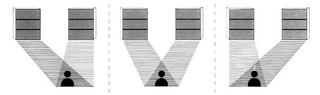
The balance can be shifted by pushing the <a href="BALANCE">BALANCE</a> slider up (less sound in the left speaker) or down (less sound in the right speaker).
