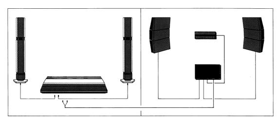
A Master Control Link 2 system can be connected to the Beomaster 3300. This enables you to operate and listen to all the units in the Beosystem 3300 in any room in your house where you have installed a Master Control Link unit.
