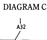
A connection to another diagram page is indicated by a number as well as by a letter of the diagram to which the connection leads.
