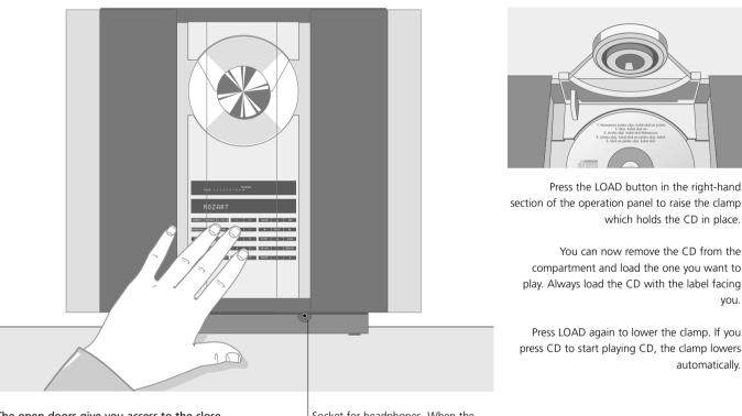
The open doors give you access to the closeup operation panel which gives you complete control of the CD player and the radio. Socket for headphones. When the headphones are plugged in, the speakers connected to BeoSound 3000 are muted.
