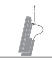
If no permanent FM aerial connection is available, an indoor aerial may be hooked onto the clamp on the back of the BeoSound 3200.
