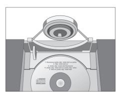
Press the LOAD button to raise the clamp which holds the CD in place.
