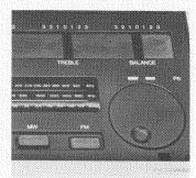
P6 may be tuned to any station of your choice in the FM, long-wave or medium-wave bands. First press P6 and thereafter either LW, MW or FM. With the large tuning knob select the station of your choice, tuning for equal brightness of the two red indicator lights.
