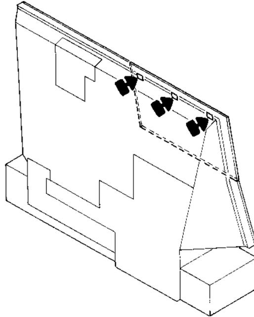
Loosen the 3 locking pins with a fine screwdriver after which the operating panel can be lifted at the front edge and pulled upwards.
