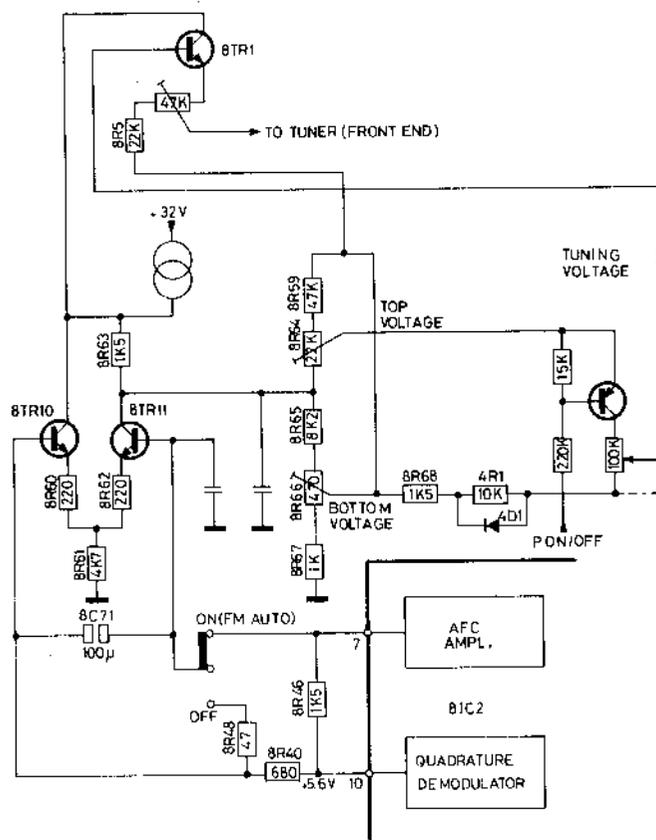
The tuning system is supplied from +32V via a constant-current generator. The bottom voltage is adjustable with 8R66 and the top voltage with 8R64.
