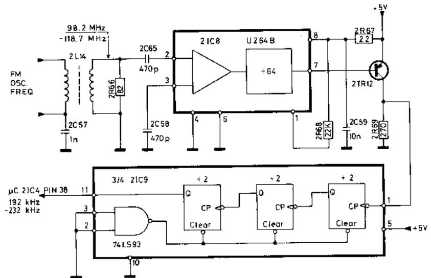
The FM oscillator frequency is being counted by the microcomputer which internally subtracts the intermediate-frequency ratio from the oscillator frequency with the result that the correct aerial frequency can be read out on the display.
