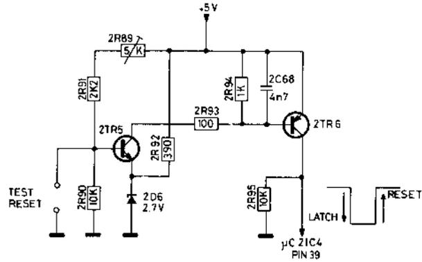
In order to inhibit the microcomputer from locking to a random internal program during start-up of the power supply or after a mains dropout of a duration of more than 1 second (cf. microcomputer power back-up), the above circuit has been incorporated.
