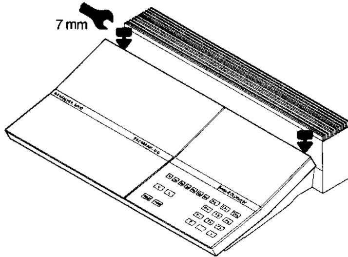
Remove the screw covers and loosen the two screws. The top part can now be lifted and put into service position.
