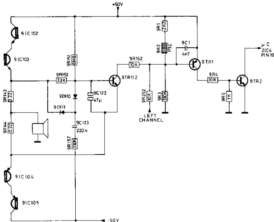
A voltage swing (a signal) on the output will charge 9C122 to a negative voltage via 9D111, 9C123, 9D110, and the resistor 9R157 which is limiting the charging.
