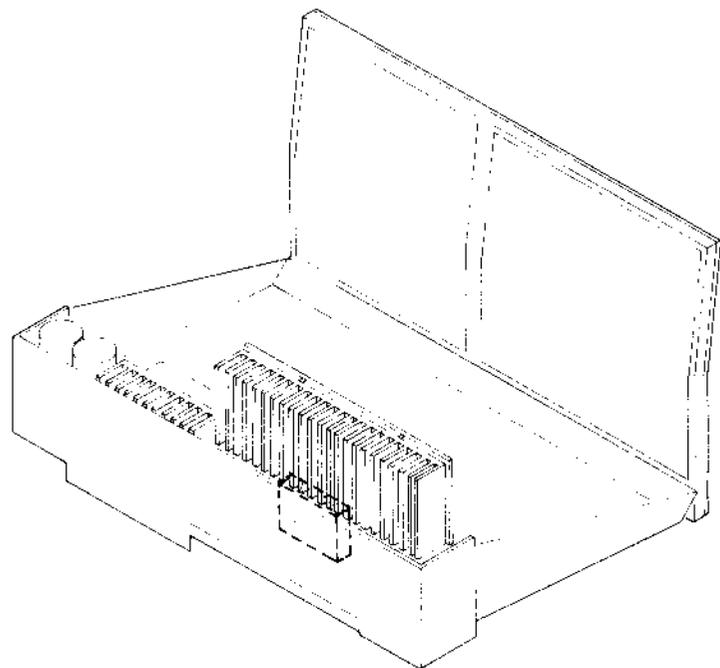
The foam block placed over the electrolytic capacitors of the power supply may be used as support during measurements in the output amplifier. The whole component side will then be accessible for measurements.
