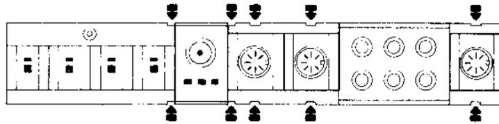
For replacement of DIN and FM sockets the terminals at the rear of the PC plate can be de-soldered and the socket clipped loose through the holes in the angle.
