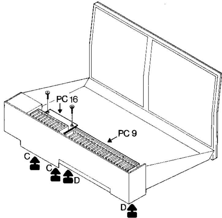
Loosen screws C and remove the two screws on top of PC16. The power supply may now be removed.
