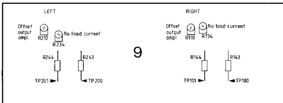
Connect a DC millivoltmeter across the two emitter resistors 9R143/9R144 (9R243/9R244) in TP100/TP101 (TP200/TP201). Adjust with 9R134 (9R234) until a reading of 22 mV is obtained.
