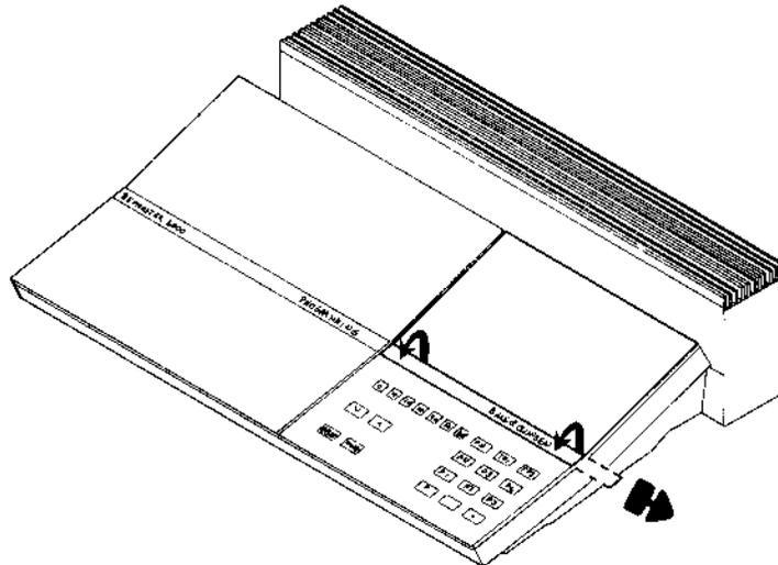
Push the decorative profile between the glass plate and the operating panel to the right and remove it. Lift the glass plate at the front edge and pull it outwards.
