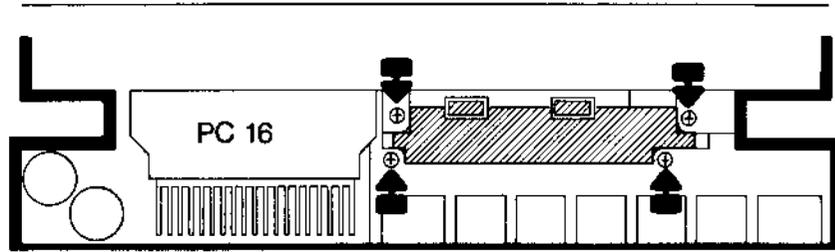
Set the top part into service position, remove the cooling grill and lift up the output amplifier. The 4 screws can now be removed.
