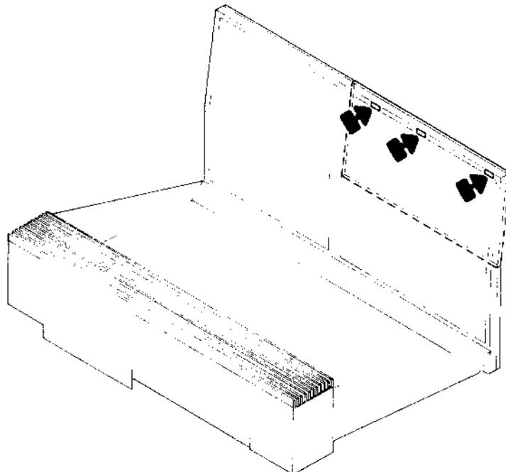
With the top part in the service position the 3 locking pins can be loosened with a screwdriver, and the panel with lid can be pulled up.
