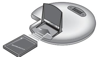
*Open the small compartment on the back of BeoSound 2 to insert the memory card.*
