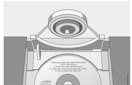
Press the LOAD button in the right-hand section of the operation panel to raise the clamp which holds the CD in place.
